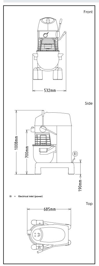
Electric Supply voltage: 600257 (XBM20AT6M) 208-230 V/1N ph/60 Hz Capacity: Performance (up to): 20 litres Capacity: **Key Information:**
